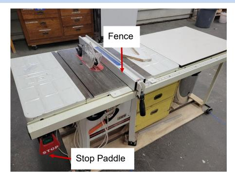
Although the table saw is one of the most useful machines in the wood shop, it is also one of the most dangerous. It can be used to accurately rip and crosscut lumber and sheet goods. The table saw can also be used for special operations including cutting dadoes and rabbets and for resawing. With the use of special jigs, joinery like tenons and box joints can be made. In addition, the blade can be tilted for cutting bevels and miters.
