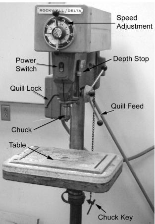
The drill press is an excellent machine for drilling accurate holes and is invaluable when drilling large holes. It consists of a motor/head assembly, chuck, and work table. Any uses other than drilling holes are special setups and must be approved by the instructor.
