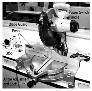
The miter or chop saw is the best tool in the lab for accurately crosscutting surfaced lumber to length. It is extremely useful for making all cuts from  $90^{\circ}$  to  $\pm 45^{\circ}$ . The miter saw is one of the most dangerous machines in the lab. Use care in its operation.
