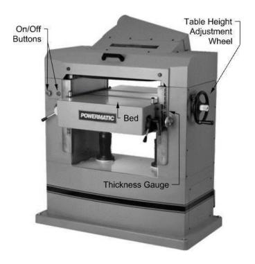
The planer is used to smooth lumber to an even thickness. After flattening one side of a board on the jointer, the board is run through the planer with the flat side down on the table, which supports the board and acts as a reference surface. The cutterhead, located above the workpiece, then smoothes the opposite face and makes it parallel to the jointed face. The width of the cutterhead, which defines the size of a planer, indicates the widest board that can be surfaced.
