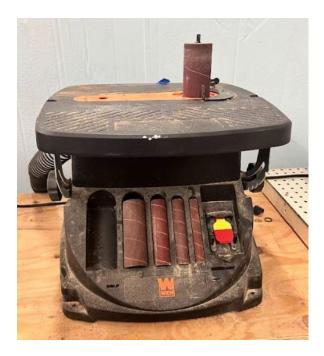
The spindle sander is used to sand inside (concave) curves. The spindle rotates while simultaneously oscillating up and down. This helps keep the abrasive from loading up and overheating, which would happen if the spindle did not move up and down. Various spindle sizes can be used on the machine to accommodate different work radii.
